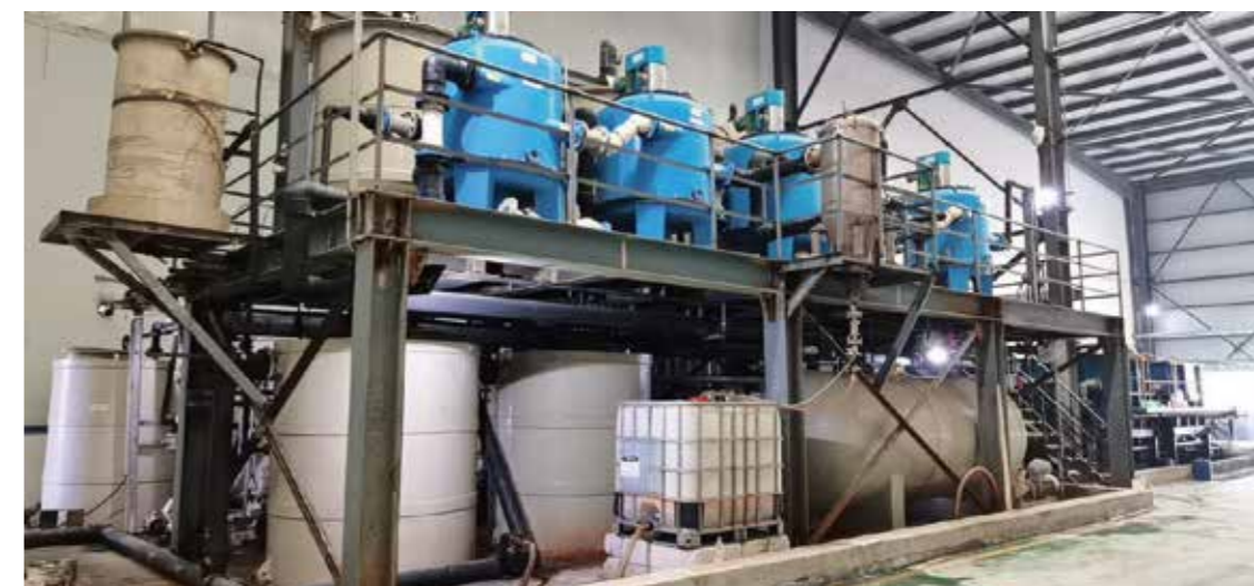
▲ Pilot test equipment for centrifugal extraction
