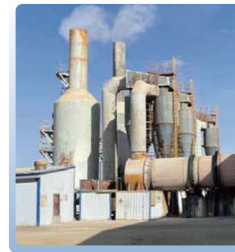
▲ Cyclone, water bath and cloth bag dust removal equipment
